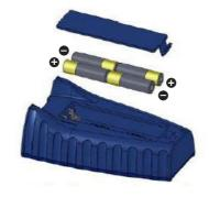
The battery compartment is located on the back of the SD 400 Oxi L device. To remove the batteries, the battery compartment lid is opened and removed. The 4 AA batteries are inserted according to the polarity. Then the battery compartment lid is replaced and closed securely.
